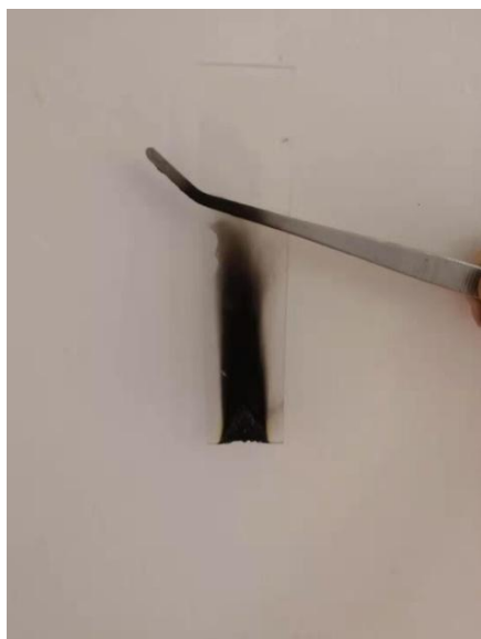
阻燃板持续点燃 30s 断开火源瞬间
